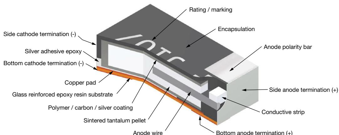
**TANTALUM CAPACITOR WITH POLYMER CATHODE TYPE T52**
