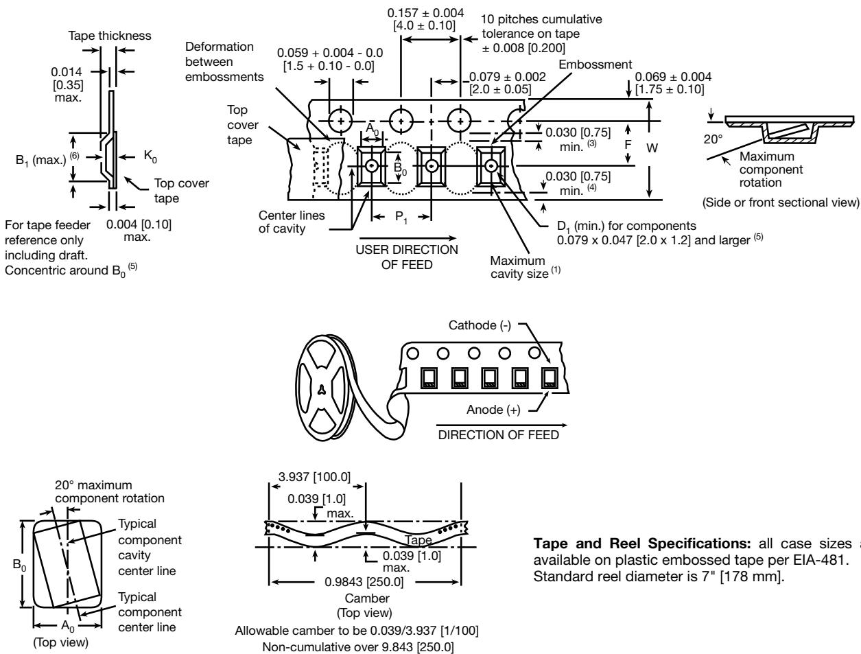
**CARRIER TAPE DIMENSIONS** in inches [millimeters]
