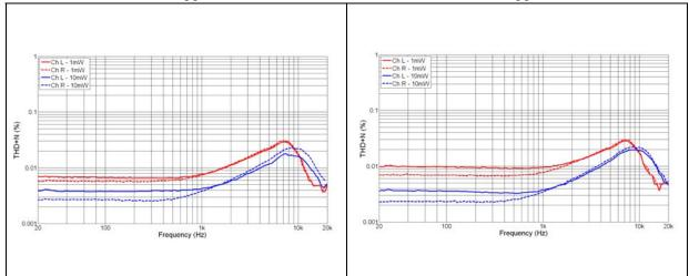
Figure 44. THD+N vs. frequency, R<sub>L</sub> = 32  $\Omega$ , out- Figure 45. THD+N vs. frequency, R<sub>L</sub> = 32  $\Omega$ , in-of-phase, V<sub>CC</sub> = 3.6 V phase, V<sub>CC</sub> = 4.8 V
