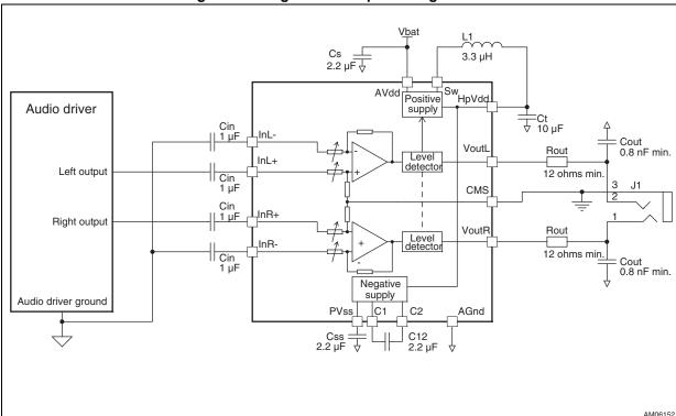
Figure 68. Single-ended input configuration1
