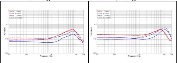
Figure 38. THD+N vs. frequency, R<sub>L</sub> = 16  $\Omega$ , outof-phase, V<sub>CC</sub> = 3.6 V Figure 39. THD+N vs. frequency, R<sub>L</sub> = 16  $\Omega$ , inphase, V<sub>CC</sub> = 4.8 V
