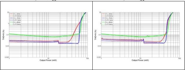
Figure 16. THD+N vs. output power - R<sub>L</sub> = 16  $\Omega$ , Figure 17. THD+N vs. output power - R<sub>L</sub> = 32  $\Omega$ , out-of-phase, V<sub>CC</sub> = 4.8 V in-phase, V<sub>CC</sub> = 2.5 V
