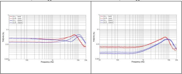
Figure 42. THD+N vs. frequency, R<sub>L</sub> = 32  $\Omega$ , out- Figure 43. THD+N vs. frequency, R<sub>L</sub> = 32  $\Omega$ , in-of-phase, V<sub>CC</sub> = 2.5 V phase, V<sub>CC</sub> = 3.6 V
