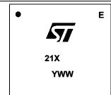
Figure 76. Flip-chip - 16 bumps
