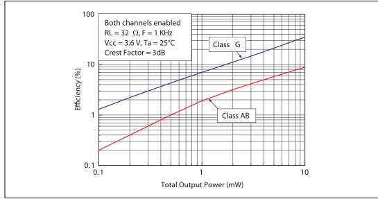
Figure 65. Efficiency comparison
