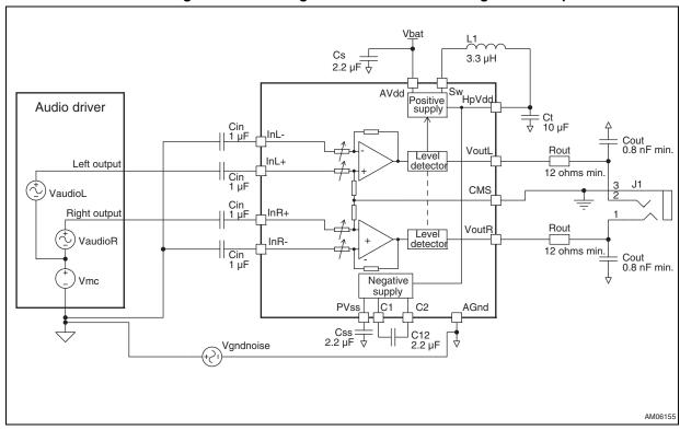
Figure 71. Correct ground connection for single-ended option
