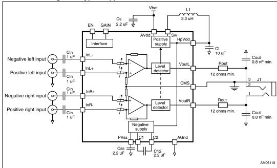
Figure 1. Typical application schematic for the A22H165
