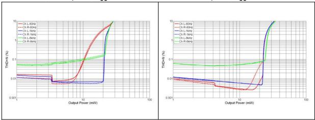
Figure 30. THD+N vs. output power - R<sub>L</sub> = 47  $\Omega$ , Figure 31. THD+N vs. output power - R<sub>L</sub> = 47  $\Omega$ , out-of-phase, V<sub>CC</sub> = 2.5 V in-phase, V<sub>CC</sub> = 3.6 V
