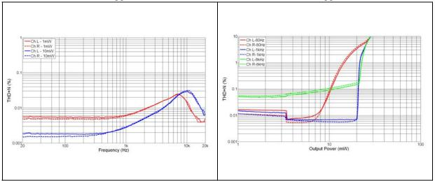
Figure 50. THD+N vs. frequency, R<sub>L</sub> = 47  $\Omega$ , out- Figure 51. THD+N vs. frequency, R<sub>L</sub> = 47  $\Omega$ , in-of-phase, V<sub>CC</sub> = 3.6 V phase, V<sub>CC</sub> = 4.8 V
