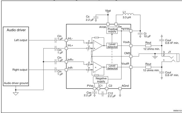
Figure 69. Single-ended input configuration 2
