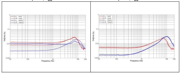
Figure 48. THD+N vs. frequency, R<sub>L</sub> = 47  $\Omega$ , out- Figure 49. THD+N vs. frequency, R<sub>L</sub> = 47  $\Omega$ , in-of-phase, V<sub>CC</sub> = 2.5 V phase, V<sub>CC</sub> = 3.6 V
