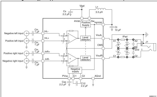
Figure 67. Typical application schematic with IEC 61000-4-2 ESD protection
