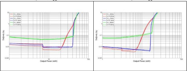
Figure 24. THD+N vs. output power - R<sub>L</sub> = 32  $\Omega$  Figure 25. THD+N vs. output power - R<sub>L</sub> = 32  $\Omega$  +IPad, out-of-phase, V<sub>CC</sub> = 2.5 V +IPad, in-phase, V<sub>CC</sub> = 3.6 V
