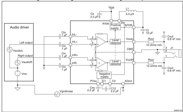
Figure 70. Incorrect ground connection for single-ended option
