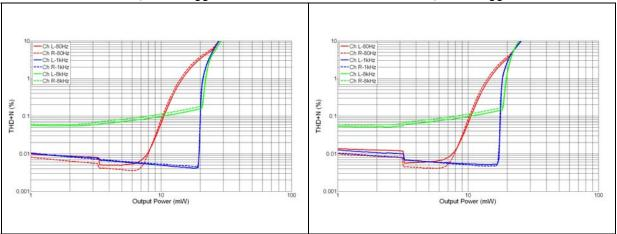
Figure 26. THD+N vs. output power - R<sub>L</sub> = 32  $\Omega$  Figure 27. THD+N vs. output power - R<sub>L</sub> = 32  $\Omega$  +IPad, out-of-phase, V<sub>CC</sub> = 3.6 V +IPad, in-phase, V<sub>CC</sub> = 4.8 V
