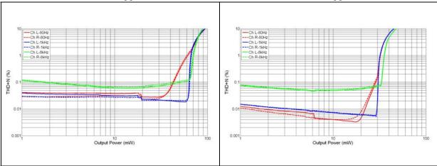
Figure 18. THD+N vs. output power - R<sub>L</sub> = 32  $\Omega$ , Figure 19. THD+N vs. output power - R<sub>L</sub> = 32  $\Omega$ , out-of-phase, V<sub>CC</sub> = 2.5 V in-phase, V<sub>CC</sub> = 3.6 V
