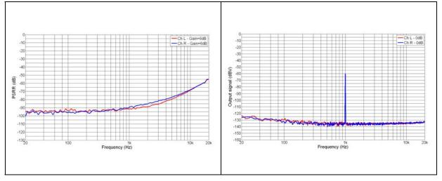
Figure 56. Crosstalk vs. frequency - R<sub>L</sub> = 32  $\Omega$ , Figure 57. Crosstalk vs. frequency - R<sub>L</sub> = 32  $\Omega$ , V<sub>CC</sub> = 3.6 V, gain = +6 dB
