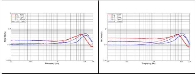
Figure 40. THD+N vs. frequency, R<sub>L</sub> = 16  $\Omega$ , out- Figure 41. THD+N vs. frequency, R<sub>L</sub> = 32  $\Omega$ , in-of-phase, V<sub>CC</sub> = 4.8 V phase, V<sub>CC</sub> = 2.5 V
