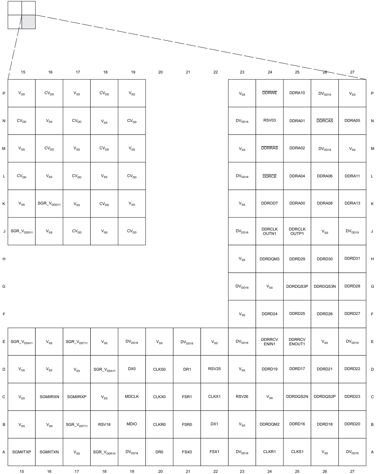
Figure 2-4. C6474 Pin Map (Bottom View) [Quadrant C]
