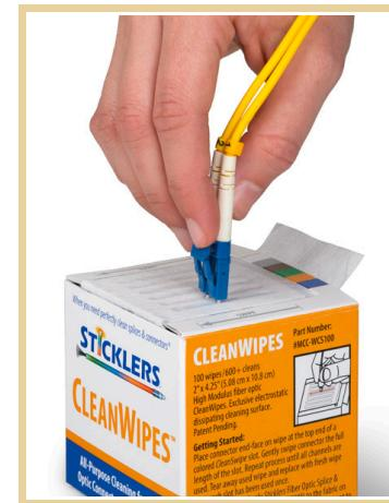
**Color-Coded slots provide six clean end-faces per wipe. Slots are spaced to clean simplex and duplex connectors with a single pass.**
