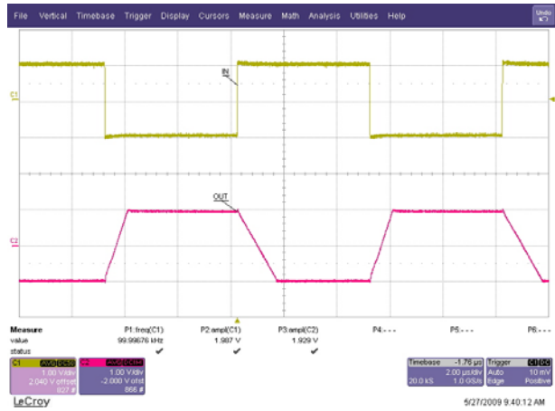
Figure 12. Inverting Large Signal Step Response
