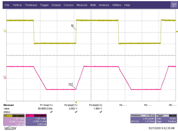
Figure 10. Non-Inverting Large Signal Step Response
