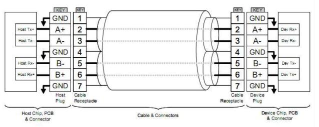
Figure 1-3 SATA Cable / Connector Connection Diagram
