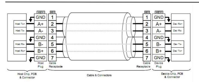
Figure 1-3 SATA Cable/Connector Connection Diagram
