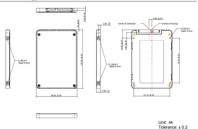
Figure 6-1 SFD25A with 7mm Housing Physical Dimensions
