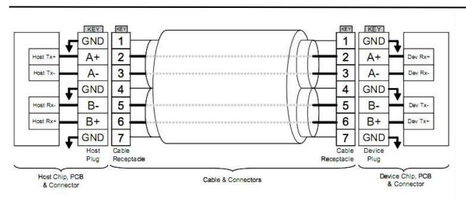
Figure 1-3 SATA Cable / Connector Connection Diagram
