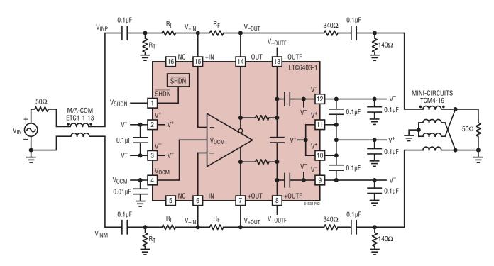
Figure 2. AC Test Circuit (-3dB BW Testing)
