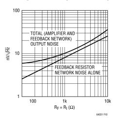
Figure 10. LTC6403-1 Output Spot Noise vs Spot Noise Contributed by Feedback Network Alone
