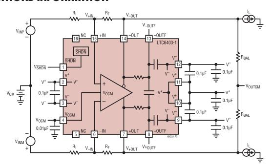
Figure 1. DC Test Circuit
