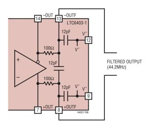
Figure 6. LTC6403-1 Internal Filter Topology
