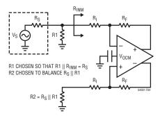
Figure 4. Optimal Compensation for Signal Source Impedance
