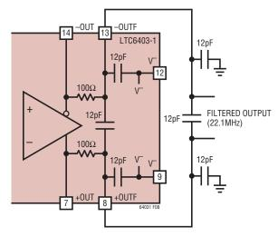
Figure 8. LTC6403-1 Filter Topology Modified for 1/2x Filter Bandwidth (3 External Capacitors)
