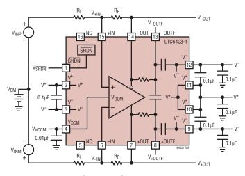
Figure 5. Circuit for Common Mode Range
