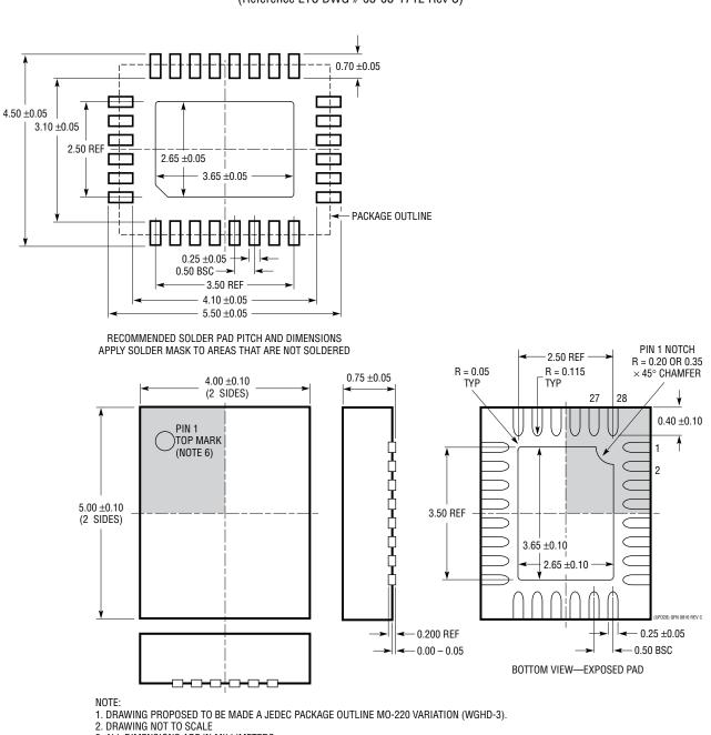
UFD Package 28-Lead Plastic QFN (4mm × 5mm) (Reference LTC DWG # 05-08-1712 Rev C)
