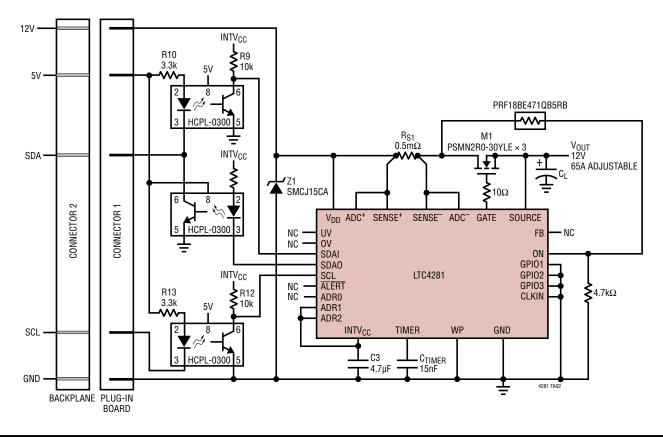
12V, 65A Application with Optical I<sup>2</sup>C Isolation and Thermal Shutdown
