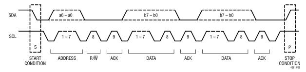
Figure 9. Data Transfer Over I<sup>2</sup>C or SMBus
