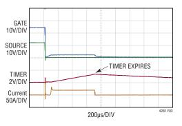
Figure 3. Short-Circuit Waveform
