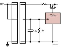
(a) ON Configured Active High (Default) CONTROL Register 0x00 Bit 5=1
