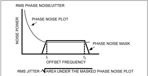
FIGURE 6-1: RMS Phase/Noise/Jitter.
