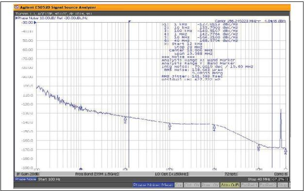
FIGURE 7-2: 156.25 MHz HCSL Output, 12 kHz to 20 MHz, 162 fs
