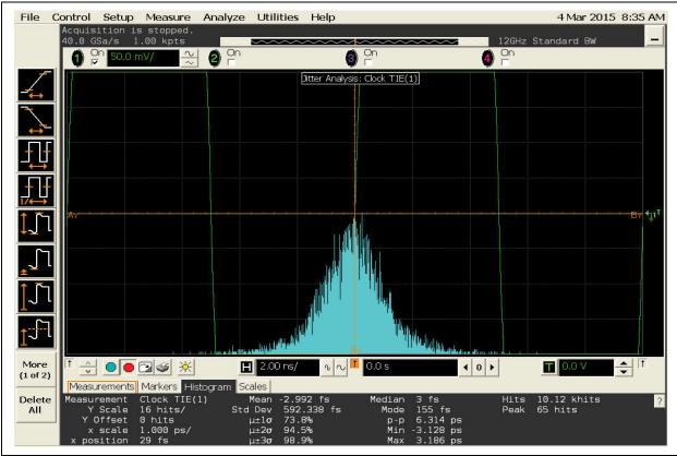
FIGURE 7-5: TIE Jitter (10k Samples).
