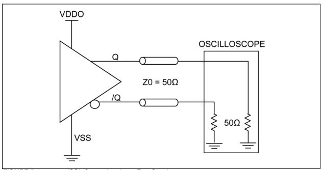
FIGURE 7-1: HCSL Output Load and Test Circuit.
