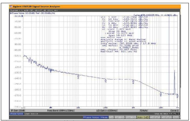
FIGURE 7-3: 156.25 MHz HCSL Output, 1.875 MHz to 20 MHz, 73 fs
