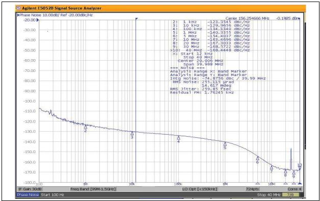
FIGURE 7-4: 156.25 MHz HCSL Output, 12 kHz to 40 MHz, 260 fs
