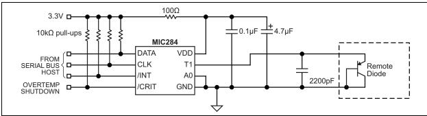
FIGURE 5-2: VDD Decoupling for very Noisy Supplies.
