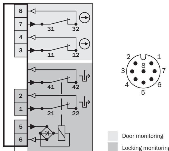
↳ Positive action N/C locking monitoring contact
