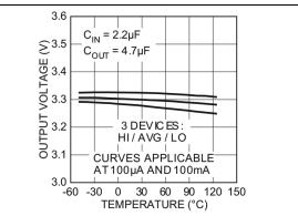
*FIGURE 2-10:* Output Voltage vs. Temperature (3.3V Version).
