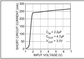
**FIGURE 2-13**: Short-Circuit Current vs. Input Voltage.
