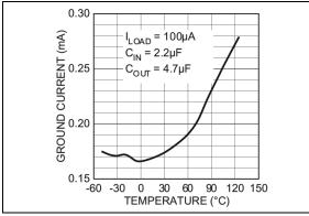
FIGURE 2-7: Ground Current vs. Temperature.
