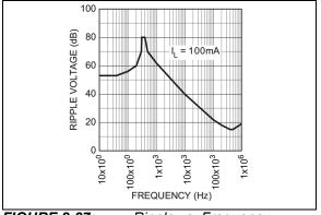
FIGURE 2-27: Ripple vs. Frequency.
