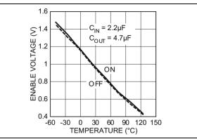
**FIGURE 2-24:** Enable Voltage Threshold vs. Temperature.
