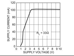
FIGURE 2-16: Supply Current vs. Supply Voltage (3.3V Version).
