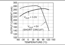
**FIGURE 2-11:** Output Current vs. Temperature.
