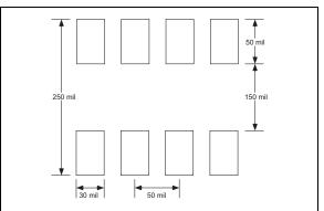
FIGURE 4-4: Minimum Recommended SOIC-8 PCB Pads Size.
