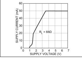
FIGURE 2-19: Supply Current vs. Supply Voltage (3.3V Version).
