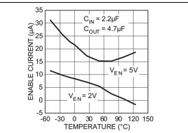
**FIGURE 2-23:** Enable Current Threshold vs. Temperature.
