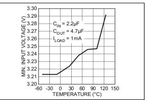
*FIGURE 2-12: Minimum Input Voltage vs. Temperature.*
