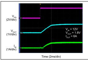
FIGURE 2-22: Enable Turn-On Delay and Rise Time.
