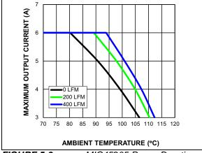
**FIGURE 5-9:** MIC45205 Power Derating vs. Airflow (24V<sub>IN</sub> to 1.5V<sub>OUT</sub>).
