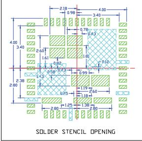
FIGURE 9-2: Solder Stencil Opening.
