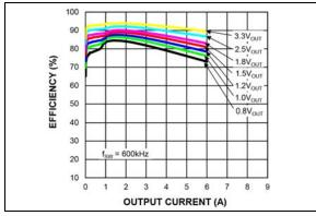
**FIGURE 2-9:** Efficiency  $(V_{IN} = 5V)$  vs. Output Current (MIC45205-1).
