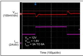
**FIGURE 2-35:** Transient Response, MIC45205-1 (I<sub>OUT</sub> = 3A to 6A).
