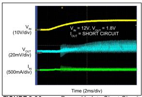
FIGURE 2-26: Power-Up Into Short-Circuit.
