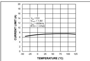
FIGURE 2-8: Output Peak Current Limit vs. Temperature.
