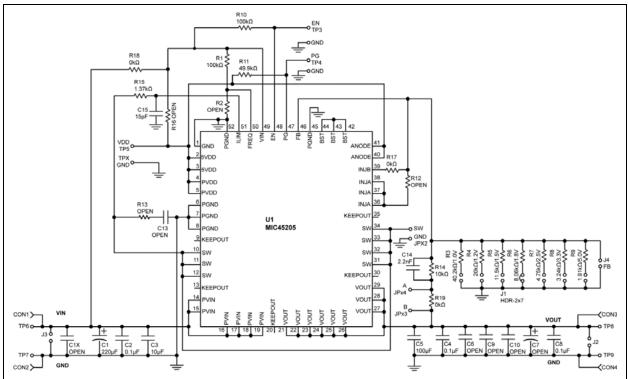
FIGURE 8-1: MIC45205YML Evaluation Board Schematic.
