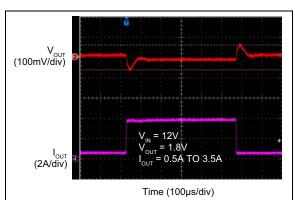
**FIGURE 2-36:** Transient Response, MIC45205-1 (I<sub>OUT</sub> = 0.5A to 3.5A).
