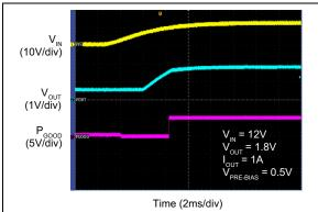
**FIGURE 2-24:** V<sub>IN</sub> Start-Up with Pre-Biased Output.
