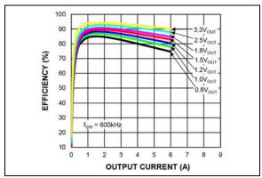
**FIGURE 2-12:** Efficiency  $(V_{IN} = 5V)$  vs. Output Current (MIC45205-2).
