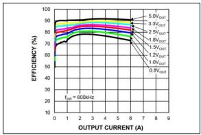
**FIGURE 2-10:** Efficiency  $(V_{IN} = 12V)$  vs. Output Current (MIC45205-1).
