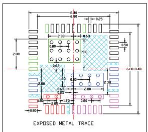
FIGURE 9-1: Exposed Metal Trace.
