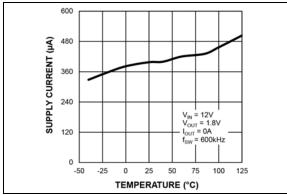
**FIGURE 2-1:** V<sub>IN</sub> Operating Supply Current vs. Temperature (MIC45205-1).
