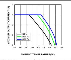
**FIGURE 5-6:** MIC45205 Power Derating vs. Airflow (5V<sub>IN</sub> to 1.5V<sub>OUT</sub>).
