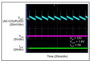
**FIGURE 2-33:** Switching Waveforms, MIC45205-1 (I<sub>OUT</sub> = 0A).
