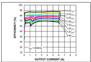
**FIGURE 2-11:** Efficiency  $(V_{IN} = 24V)$  vs. Output Current (MIC45205-1).
