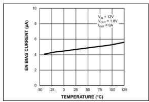
FIGURE 2-4: EN Bias Current vs. Temperature.
