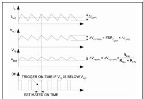
FIGURE 4-2: MIC45205 Control Loop Timing.
