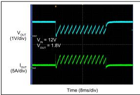
FIGURE 2-29: Output Recovery from Short-Circuit.
