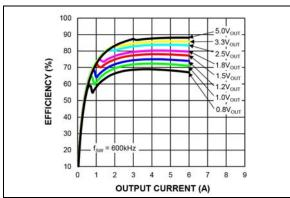
**FIGURE 2-14:** Efficiency  $(V_{IN} = 24V)$  vs. Output Current (MIC45205-2).
