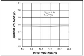
**FIGURE 2-16:** Output Voltage vs. Input Voltage.
