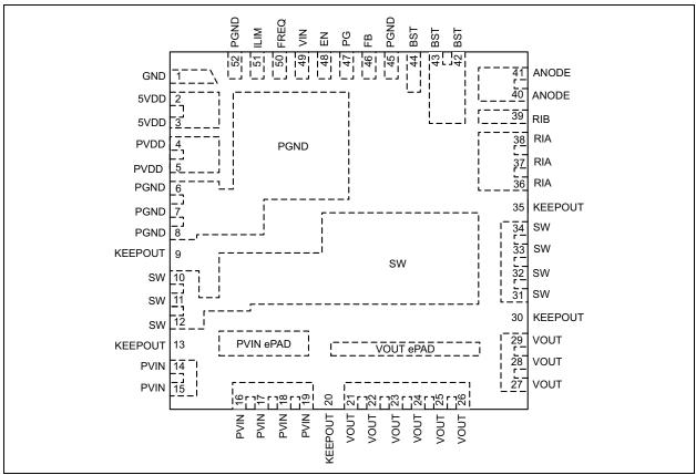
FIGURE 3-1: MIC45205 Pin Configuration.
