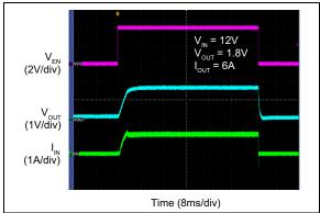
**FIGURE 2-34:** Inrush with  $C_{OUT} = 3000 \mu F$ .
