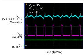
**FIGURE 2-32:** Switching Waveforms ( $I_{OUT} = 6A$ ).
