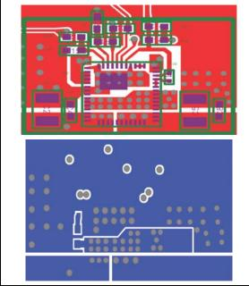
FIGURE 6-1: Top And Bottom Layer of a Four-Layer Board.
