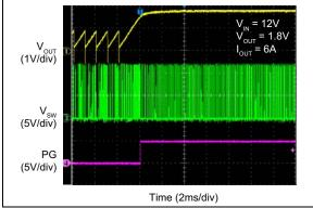
FIGURE 2-31: Output Recovery from Thermal Shutdown.
