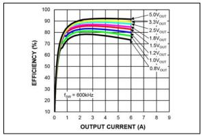
FIGURE 2-13: Efficiency  $(V_{IN} = 12V)$  vs. Output Current (MIC45205-2).
