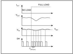
**FIGURE 4-3:** MIC45205 Load Transient Response.
