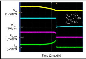
FIGURE 2-21: V<sub>IN</sub> Soft Turn-Off.
