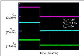
FIGURE 2-23: Enable Turn-Off Delay and Fall Time.
