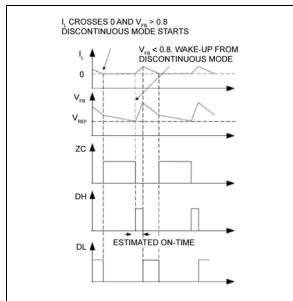
FIGURE 4-4: MIC45205-1 Control Loop Timing (Discontinuous Mode).
