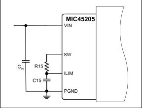
FIGURE 4-5: MIC45205 Current-Limiting Circuit.
