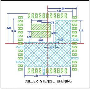
FIGURE 7-2: Solder Stencil Opening.
