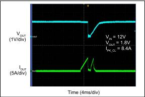
FIGURE 2-30: Peak Current-Limit Threshold.
