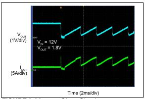
FIGURE 2-28: Short-Circuit.
