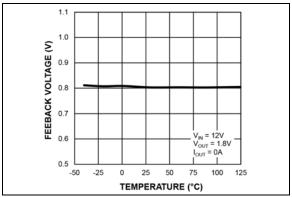
**FIGURE 2-5:** Feedback Voltage vs. Temperature.
