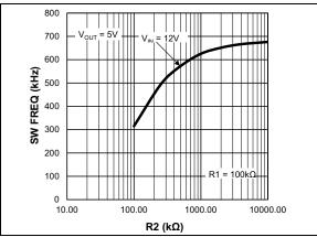
FIGURE 5-2: Switching Frequency vs. R2.
