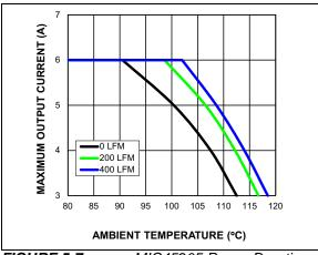
**FIGURE 5-7:** MIC45205 Power Derating vs. Airflow (12V<sub>IN</sub> to 1.5V<sub>OUT</sub>).
