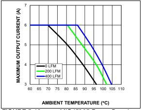
**FIGURE 5-10:** MIC45205 Power Derating vs. Airflow (24V<sub>IN</sub> to 3.3V<sub>OUT</sub>).
