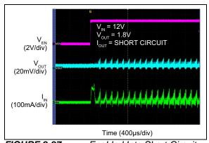
FIGURE 2-27: Enabled Into Short-Circuit.
