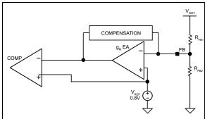
FIGURE 4-1: Output Voltage Sense via FB Pin.
