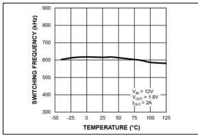
**FIGURE 2-7:** Switching Frequency vs. Temperature.
